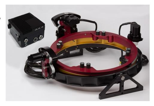
Contrary to other mount designs, the STX open circular gimbal allows the sensor system to be fixed to the mount so as to be as low as possible above the airplane hole. As the center of rotation is also located as low as possible, the sensor can take full advantage of the +/-14 degrees full range of correction in pitch and roll and +/-29 degrees of drift correction.
