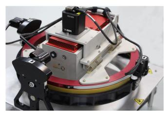
Mount with Leica RCD30 and Riegl 680i
